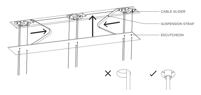
With the ESCUTCHEON in place, make any necessary final adjustments to the PENDANT.
