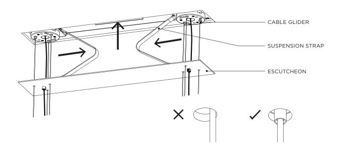
With the ESCUTCHEON in place, ensure the CORD GRIPS are adequately tightened on to the POWER CABLE and make any necessary final adjustments to the PENDANT.
