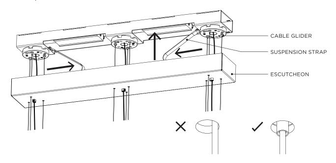
With the ESCUTCHEON in place, ensure the CORD GRIPS are adequately tightened on to the POWER CABLE and make any necessary final adjustments to the PENDANT.
