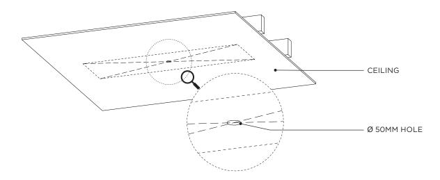
Installer to provide adequate load-bearing substrate, utilising ceiling joist where additional support is required. For accurate placement of Cable Exits in the Substrate, use the PSM as a guide.
