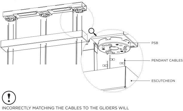
RESULT IN AN ELECTRICAL FAULT & CAUSE PRODUCT FAILURE.
