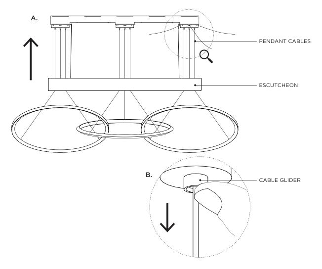
Connect the labelled PENDANT CABLES to the PSU. Refer to supplied WIRING DIAGRAM  $\rightarrow$
