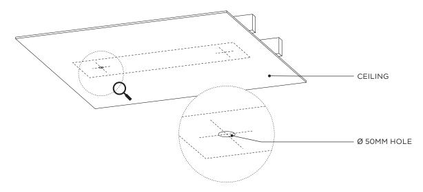
Installer to provide adequate load-bearing substrate, utilising ceiling joist where additional support is required. For accurate placement of Cable Exits in the Substrate, use the PSM as a guide.
