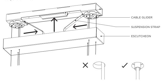
With the ESCUTCHEON in place, make any necessary final adjustments to the PENDANT.
