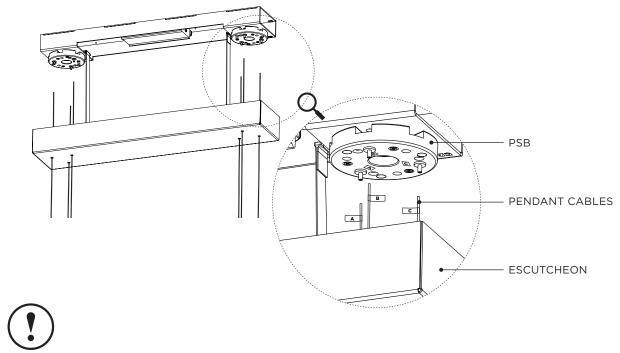
INCORRECTLY MATCHING THE CABLES TO THE GLIDERS WILL RESULT IN AN ELECTRICAL FAULT & CAUSE PRODUCT FAILURE.
