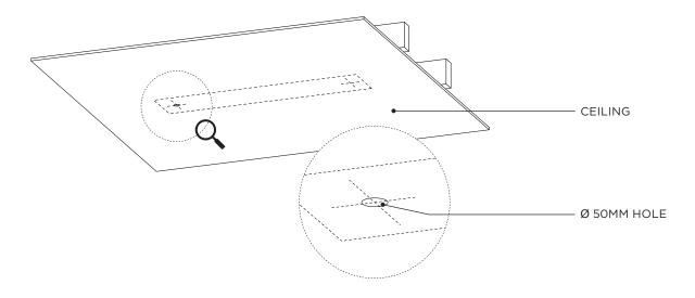
Installer to provide adequate load-bearing substrate, utilising ceiling joist where additional support is required. For accurate placement of Cable Exits in the Substrate, use the PSM as a guide.
