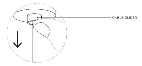
Carefully raise ESCUTCHEON to the ceiling until the Magnets engage. Ensure no contact between ESCUTCHEON and CABLE GLIDER, as this may release the suspension wire.
