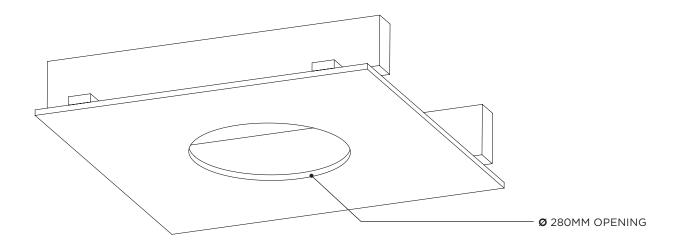
Installer to provide adequate load-bearing substrate, utilising ceiling joists where additional support is required. The mounting face of the substrate must be set back 75mm from the ceiling facade. For accurate placement of Cable Exits in the Substrate, use the PSM as a guide.
