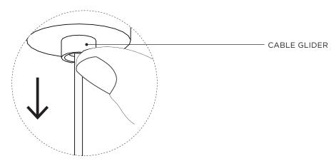
Raise ESCUTCHEON to the ceiling carefully until the Magnets engage. Ensure no contact between ESCUTCHEON and CABLE GLIDERS, as this may release the pendant cables.
