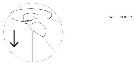
Raise ESCUTCHEON to the ceiling carefully until the Magnets engage. Ensure no contact between ESCUTCHEON and CABLE GLIDERS, as this may release the suspension wires.
