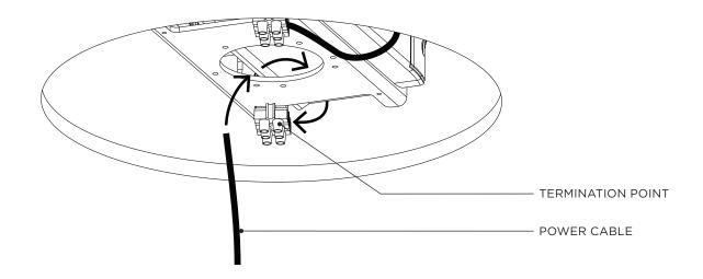
Attach the PSB to the PSM with the 3 provided COUNTERSUNK M4 FASTENERS.
