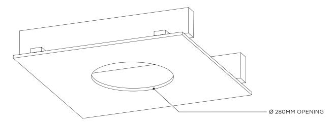
Installer to provide adequate load-bearing substrate, utilising ceiling joists where additional support is required. The mounting face of the substrate must be set back 75mm from the ceiling facade.
