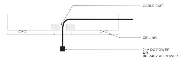
Feed the 24V Power Supply cable OR the 120-240V AC Power cable through the central hole of the PSB and attach the PSB to Substrate with appropriate Fasteners. Make sure to align the CABLE GLIDERS with the SUSPENSION WIRE EXIT HOLES.
