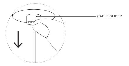
Raise ESCUTCHEON to the ceiling carefully until the Magnets engage. Ensure no contact between ESCUTCHEON and CABLE GLIDERS, as this may release the suspension wire.
