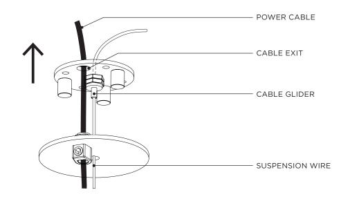
Connect the 24V DC or 110-240V AC POWER to the POWER CABLE. Refer to supplied WIRING DIAGRAM  $\rightarrow$
