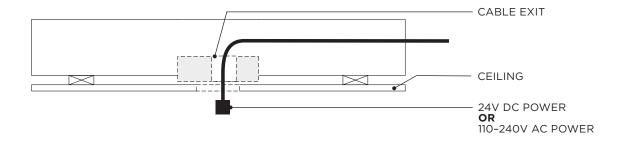
5 From the pendant, feed the SUSPENSION WIRE through central hole in the ESCUTCHEON and POWER CABLE through the CORD GRIP as shown.
