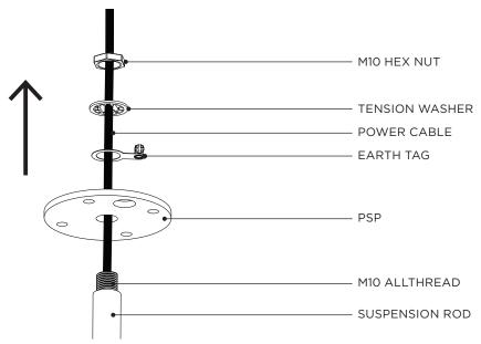
Connect the 24V DC or 110-240V AC POWER to the POWER CABLE. Refer to supplied WIRING DIAGRAM →
