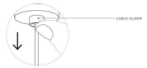
Carefully raise ESCUTCHEON to the ceiling until the Magnets engage. Ensure no contact between ESCUTCHEON and CABLE GLIDERS, as this may release the suspension wires.
