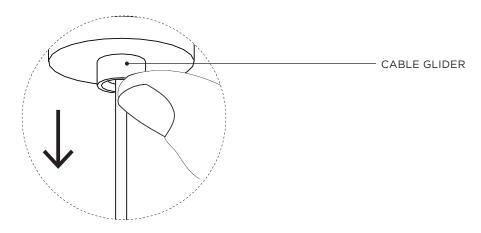
Carefully raise ESCUTCHEON to the ceiling until the Magnets engage. Ensure no contact between ESCUTCHEON and CABLE GLIDERS, as this may release the pendant cables.
