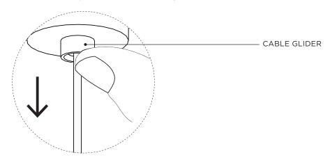
Carefully raise ESCUTCHEON to the ceiling until the Magnets engage. Ensure no contact between ESCUTCHEON and CABLE GLIDERS, as this may release the suspension wires.
