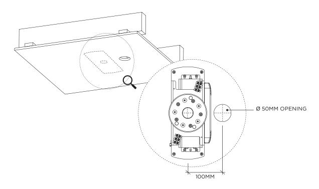
Installer to provide adequate load-bearing substrate, utilising ceiling joist where additional support is required.
