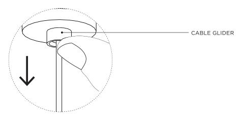
Carefully raise ESCUTCHEON to the ceiling carefully until the Magnets engage. Ensure no contact between ESCUTCHEON and CABLE GLIDERS, as this may release the pendant cables.
