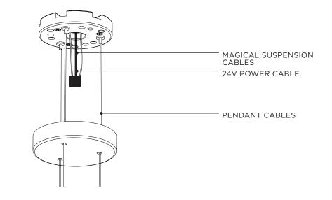
Raise the PENDANT, feeding excess cable through the CABLE GLIDERS. Set into position by gently lowering the PENDANT.
