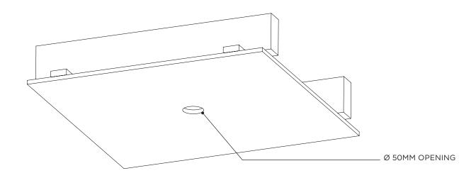
Installer to provide adequate load-bearing substrate, utilising ceiling joist where additional support is required.
