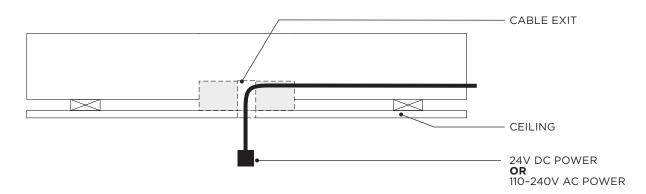
Attach the PSB to Substrate with appropriate Fasteners and feed the 24V Power Supply cable OR the 120-240V AC Power cable through the centre.
