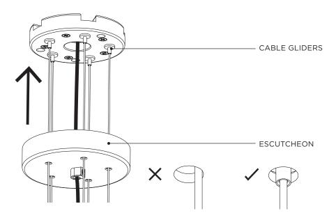
With the ESCUTCHEON in place, ensure the CORD GRIP is adequately tightened on to the POWER CABLE and make any necessary final adjustments to the PENDANT.
