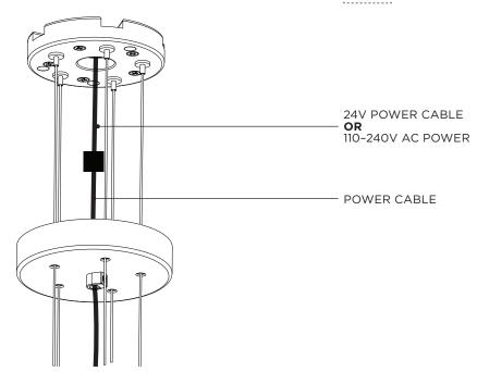
**9** Raise the PENDANT, feeding excess cable through the CABLE GLIDERS. Set into position by gently lowering the PENDANT.
