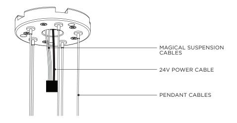
Raise the PENDANT, feeding excess cable through the CABLE GLIDERS. Set into position by gently lowering the PENDANT.
