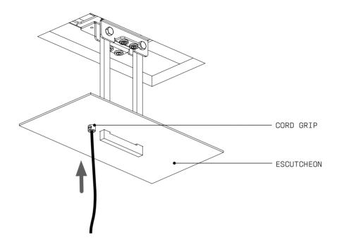
Carefully raise the ESCUTCHEON toward the PSM, until the MAGNETS engage, ensuring not to catch
