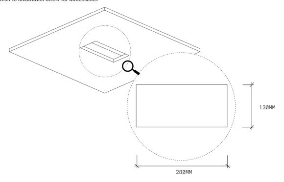
3 Installer to provide adequate load-bearing substrate, utilising ceiling joists where additional support is required. The mounting face of the substrate must be set back 90mm from the ceiling. For accurate placement of Cable Exits in the Substrate, use the PSM as a guide.
