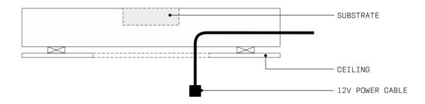
$\frac{5}{2}$  Attach the U-LINK BRACKETS to the prepared SUBSTRATE via the pilot holes with appropriate SCREW FASTENERS.
