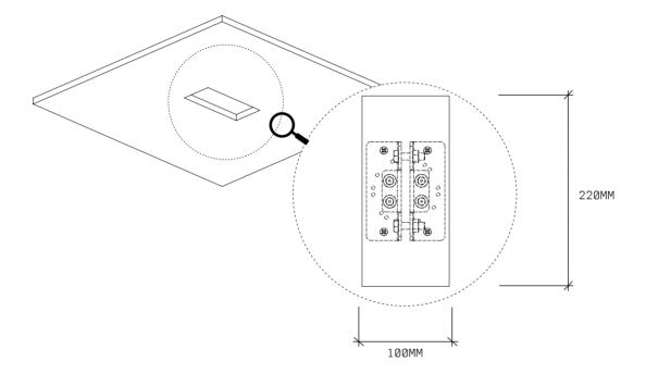
3 Installer to provide adequate load-bearing substrate, utilising ceiling joists where additional support is required. The mounting face of the substrate must be set back 40mm from the ceiling facade.
