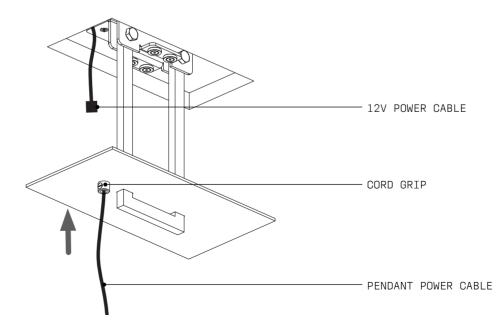
8 Carefully raise the ESCUTCHEON toward the U-LINK BRACKETS, until the MAGNETS engage, ensuring not to catch the POWER CABLE.
