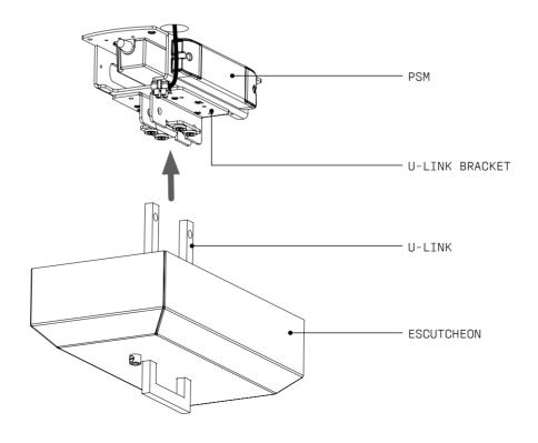
Pass the fixture cable through the CORD GRIP in the ESCUTCHEON and connect it to the PSM.
