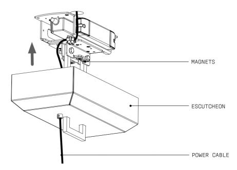
With the ESCUTCHEON in place, ensure the CORD GRIP is adequately secured on to the POWER
