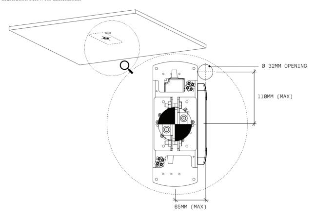
$\frac{3}{-} \quad \text{Installer to provide adequate load-bearing substrate utilising ceiling joist where additional support is required.}$
