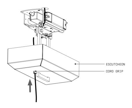
Carefully raise the ESCUTCHEON toward the PSM, until the magnets engage, ensuring not to catch
