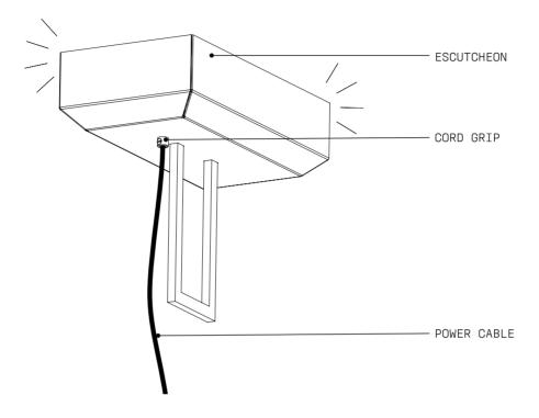
Conduct a final visual assessment of both the canopy and fixture to ensure all parts have been properly fitted and secured. Once satisfied that everything is in working order, remove all remaining protective material which will complete the installation process.
