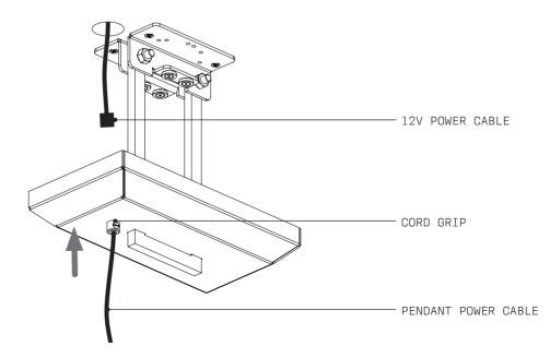
8 Carefully raise the ESCUTCHEON toward the U-LINK BRACKETS, until the MAGNETS engage, ensuring not to catch the POWER CABLE.
