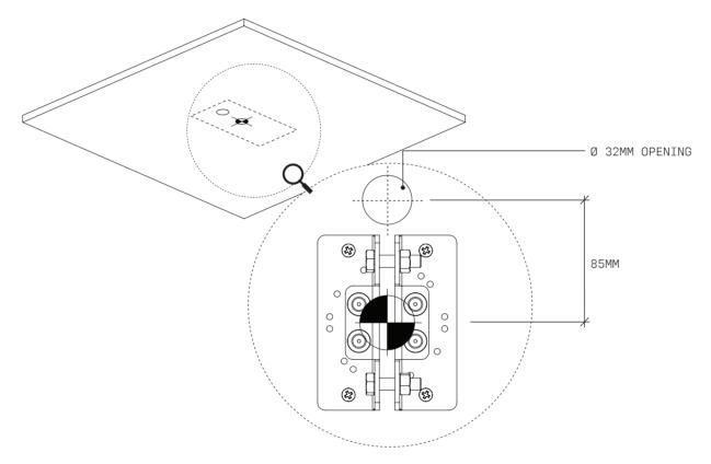
$\frac{3}{-} \quad \text{Installer to provide adequate load-bearing substrate utilising ceiling joist where additional support is required.}$
