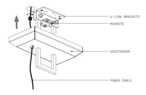
With the ESCUTCHEON in place, ensure the CORD GRIP is adequately secured on to the POWER
