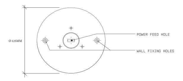
$2 \qquad \text{Remove WALL MOUNT MODULE and cut POWER FEED HOLE.} \\$
