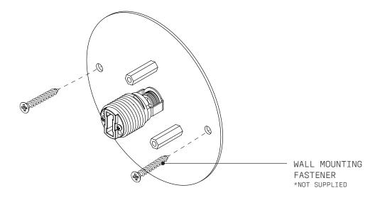
5 With the WALL MOUNT MODULE installed, align and fit the QUARTZ SLICE with the three brass screw fasteners, ensure not to scratch or mark the disc. Insert the lamp and power on to ensure correct working order.
